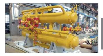
final cleaning of moisture occurs by a swirler and separating elements. The purified gas passes from separator through the outlet pipeline, on which a gas meter is installed; after measuring the gas can be directed to a flare system or gas collector.
